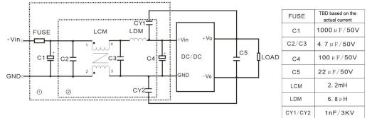
Note - part () circuit is for EMS test, (2) for EMI filtering, both can be adjusted according to acutal situation.
